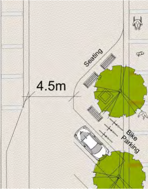
Figure 3.19: Proposed layout for section of Argyle Street with seating, bike parking and angled vehicle parking
